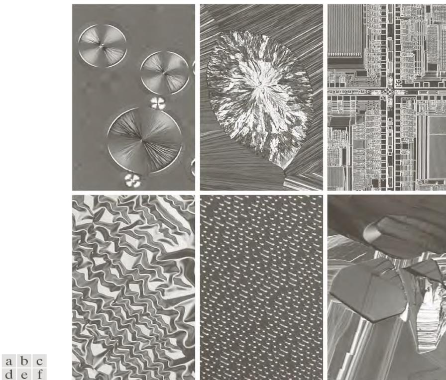
**FIGURE 1.9** Examples of light microscopy images. (a) Taxol (anticancer agent), magnified 250 $\times$ . (b) Cholesterol—40 $\times$ . (c) Microprocessor—60 $\times$ . (d) Nickel oxide thin film—600 $\times$ . (e) Surface of audio CD—1750 $\times$ . (f) Organic superconductor—450 $\times$ . (Images courtesy of Dr. Michael W. Davidson, Florida State University.)
